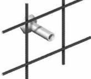
SKS24 Threaded Anchor, Part of ESDQ-L20W
