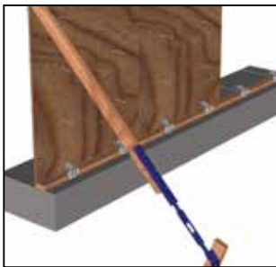
4: Place Snapties through pre-drilled panels from inside of form.
